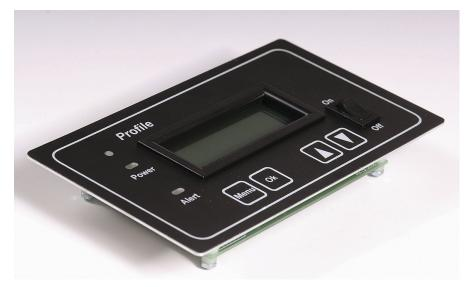
when the tank is either too high (as in a waste tank) or too low (fresh tank). The Profile Solo panel also runs the EZ-Profile software algorithm correcting for odd tank geometry and sensor type for maximum accuracy.
